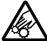
Warning, drive train
